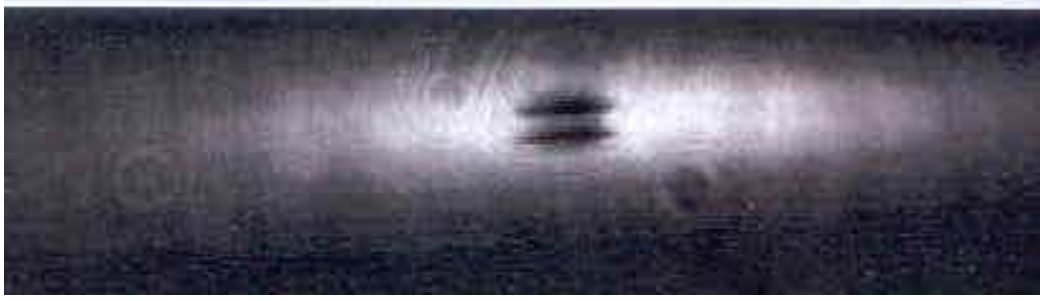
Figure 4.6: Absorption image of the atoms using 780nm imaging light passing through the same fiber as the big lattice beam
