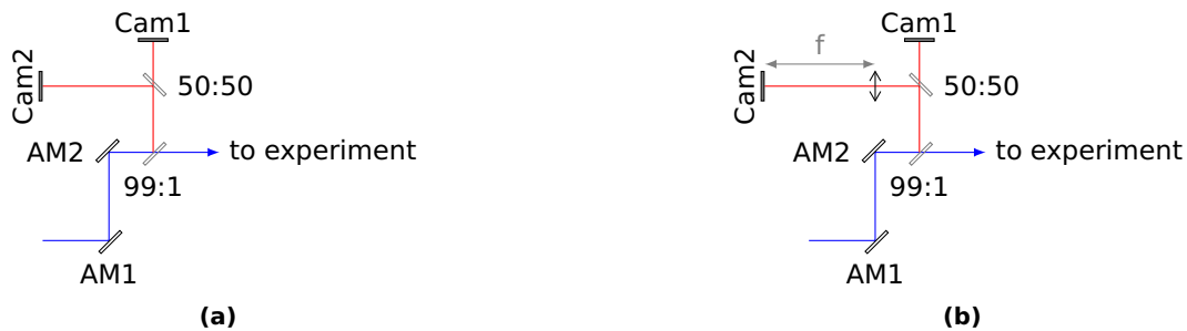
Figure A.1. Different implementations for the beam steering. AM1 and AM2 are two piezo-motor actuated automated mirrors.
